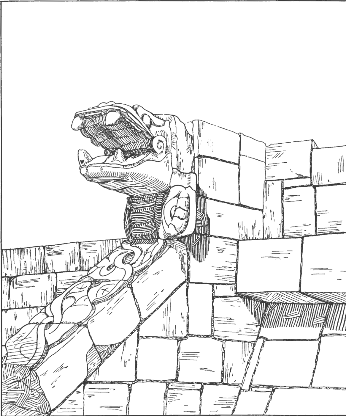
FIG. 80—PERSPECTIVE DRAWING OF SERPENT HEAD AT TOP OF SOUTH BALUSTRADE, LOWER PLATFORM STAIRWAY.
